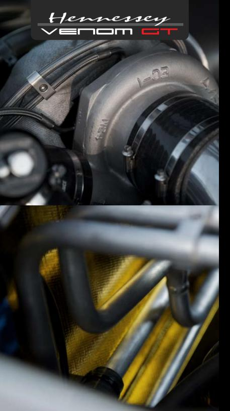
Powering the Venom GT is a 6.2L supercharged LS9 V-8 engine producing 725 bhp at 7,200 rpm.
